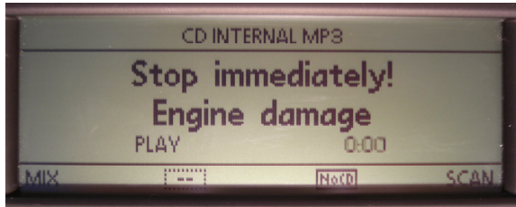
Fig. 3. Exemplary low-tech attack on multimedia system interfaces
